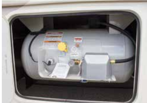
Typical propane gas tank
