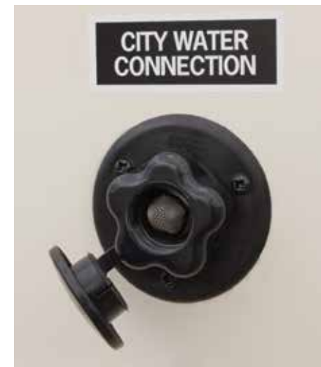
Typical city water fill
